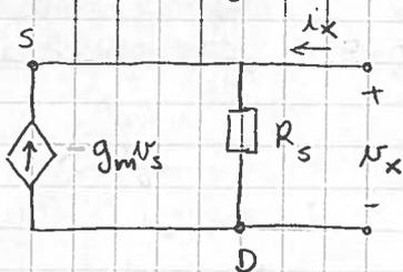
$$\text{KCL: } -g_m v_s + i_x = \frac{v_x}{R_s}$$
