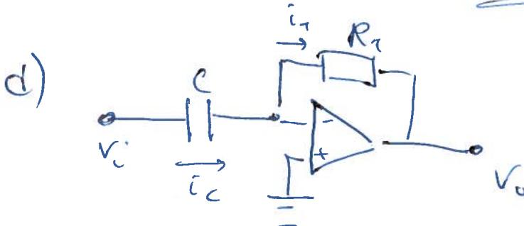
$$V_- = V_T = 0 \quad i_- = i_o$$
