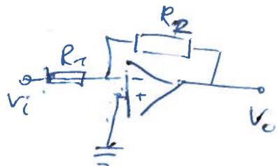
$$V_- = V_+ = 0, i_- = i_+ = 0$$
