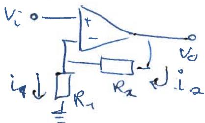
$$i_1 = \frac{V_i}{R_1}, \quad i_2 = \frac{V_o}{R_2 + R_1} = \frac{V_i}{R_1} = \frac{V_i}{R_1}$$
