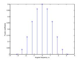
**Figure 4:** The Fourier coefficients  $c_k$  of z(n) for k = -5, ..., 5
