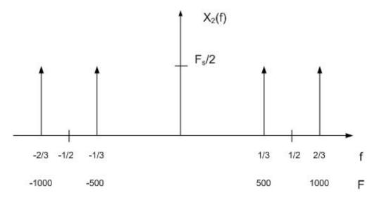
Figure 8: Spectrum of the signal x(n) when  $F_s = 1500$ Hz
