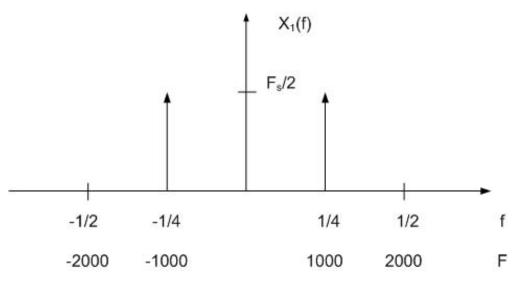
Figure 7: Spectrum of the signal x(n) when  $F_s = 4000$ Hz
