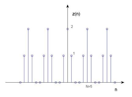
**Figure 3:** The signal z(n), periodic extension of x(n)
