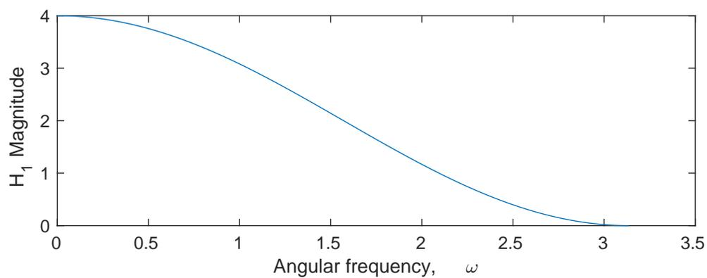
Figur 5: Amplituderrespons for  $H_1$
