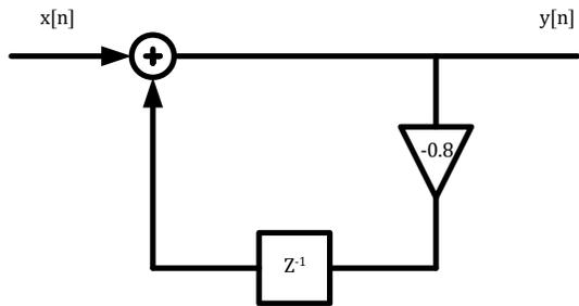
Figure 8: Filter structure of the second system
