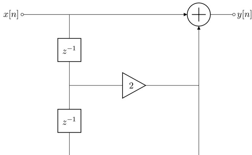
Figure 6: Filter structure of  $y_1[n] = x[n] + 2x[n - 1] + x[n - 2]$ .
