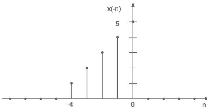
Figure 3: Flipped signal,  $x(-n)$ .
