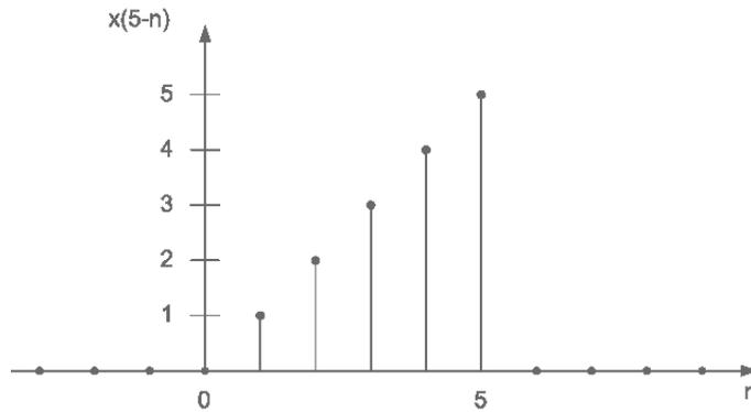
Figure 4: Flipped and shifted signal,  $x(5 - n)$ .
