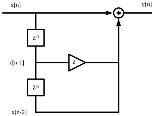
Figure 7: Filter structure of the first system
