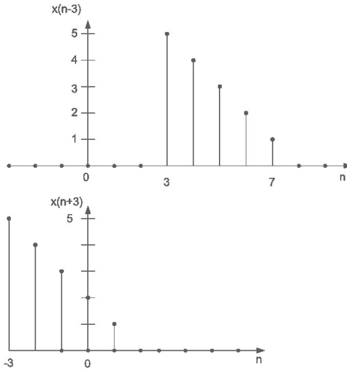
Figure 2: Shifted signals,  $x(n - 3)$  and  $x(n + 3)$ .
