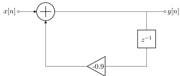
Figure 7: Filter structure of  $y_2[n] = -0.9y[n - 1] + x[n]$ .
